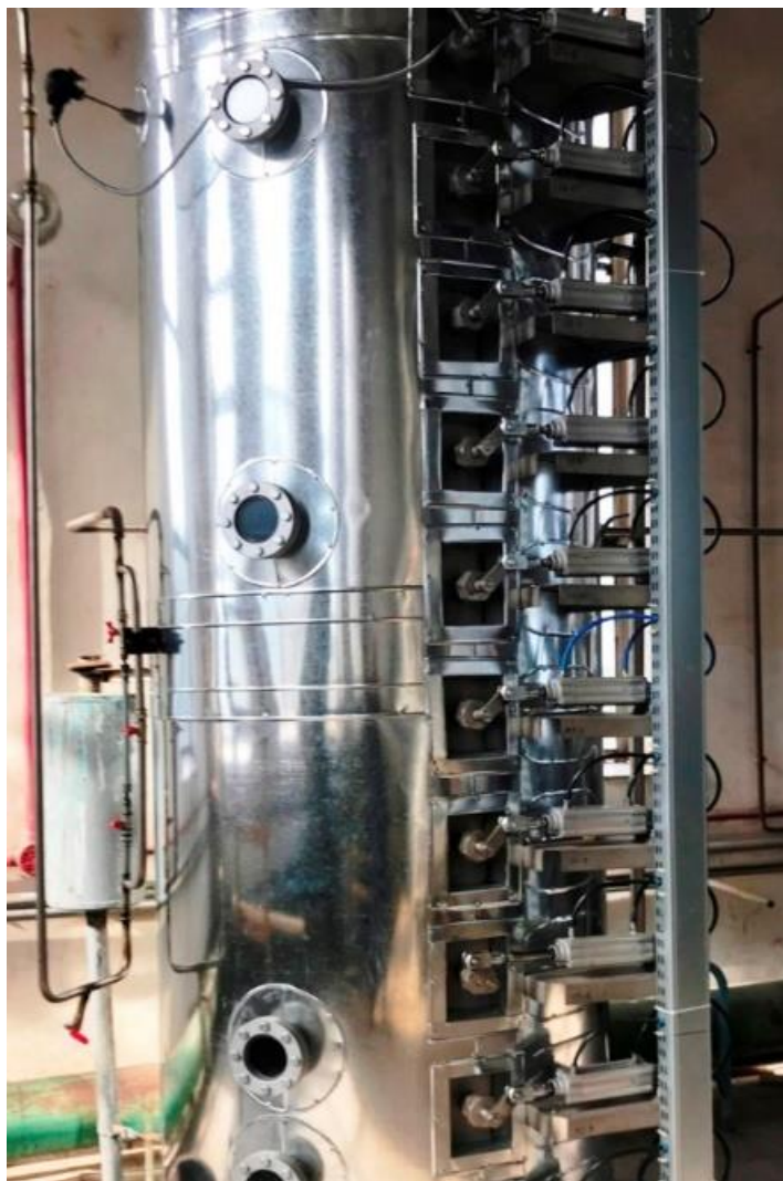
Figure 2. Experimental cyclic column with perforated plates
